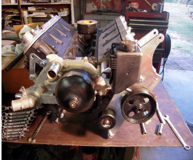
If you're using a F-body engine and you have the original power steering pump, all you have to do is remove the plastic reservoir by driving off two spring clips and giving the reservoir a good tug. You'll see a plastic sleeve that may come off with the reservoir or may stay in the pump. The sleeve may also have an o-ring. Pull out the sleeve and you'll be ready for the instructions below.
