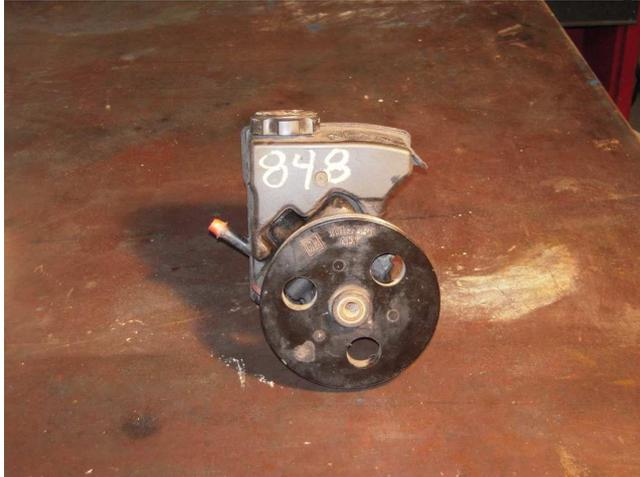
And here's one that looks completely different because of the attached plastic reservoir but the pump body is identical. This one is from a 2005 GMC Envoy (same as Chevy Trailblazer):
